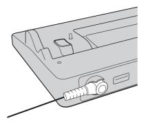
4 Remove the port replicator connector cover from the bottom of the computer.
